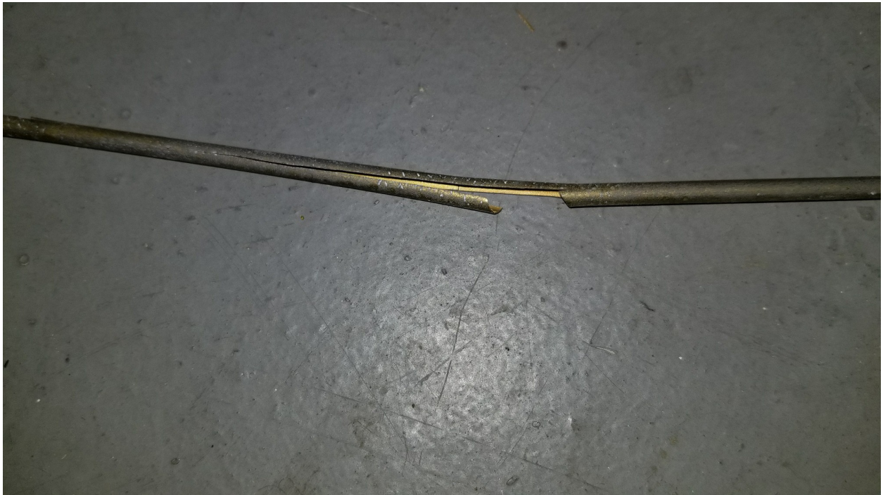
Illustration 2: Disassembly of the antenna reveals the source of "Snap, Crackle..."
