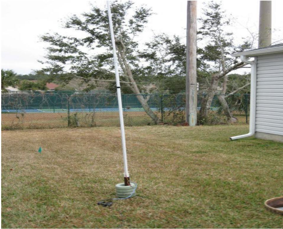
NZ1D's Q'nD inverted "L" antenna made from assorted scrap pvc and a handfull of #22 wire scavenged from Xmas lights. (NZ1D photo)
