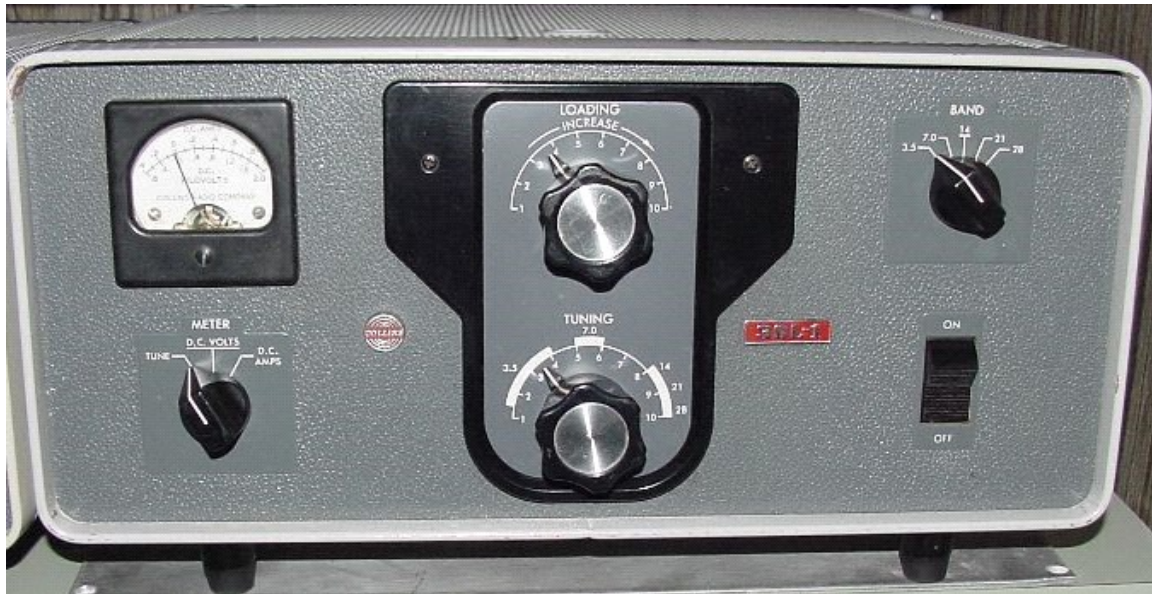
The 30L-1, table top amp, 38 pounds and runs on 115/230 VAC.
