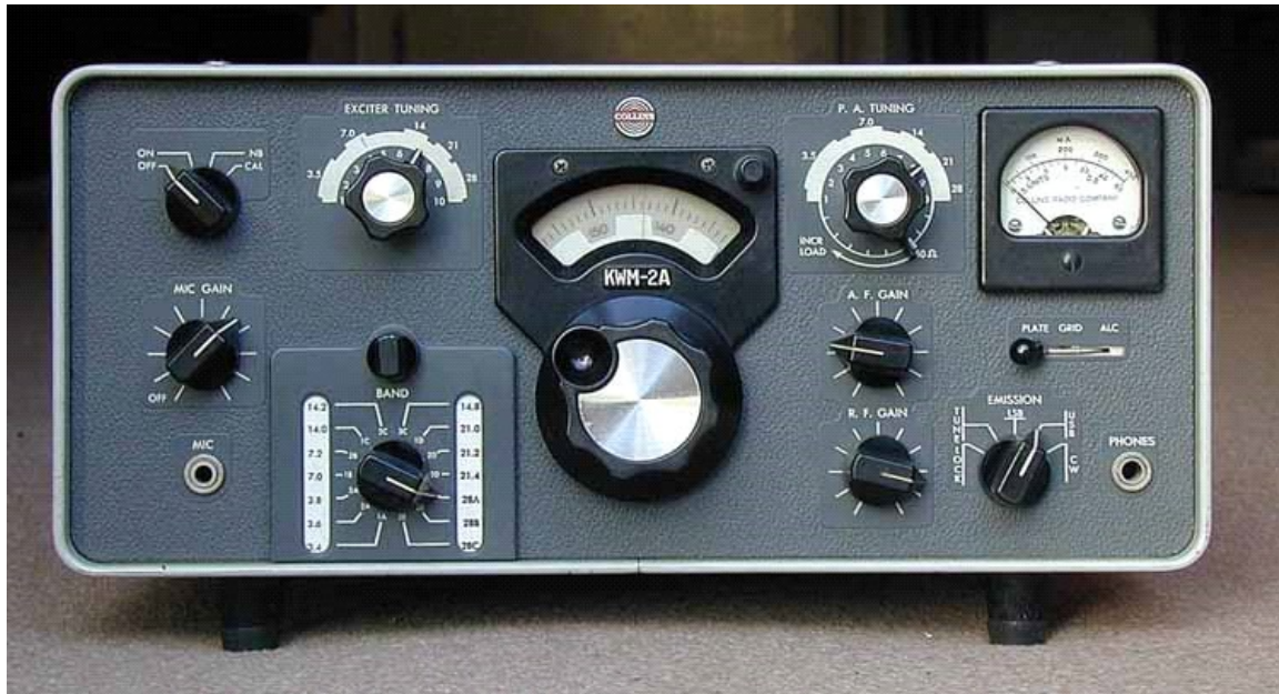
KWM-2A with addition band selection bezel and switch. When the switch was turned, a second set of blank windows appeared for the user to add frequencies outside of the ham bands, determined by added crystals under the chassis. Yours truly has one of these on "permanent loan" from its owner.
