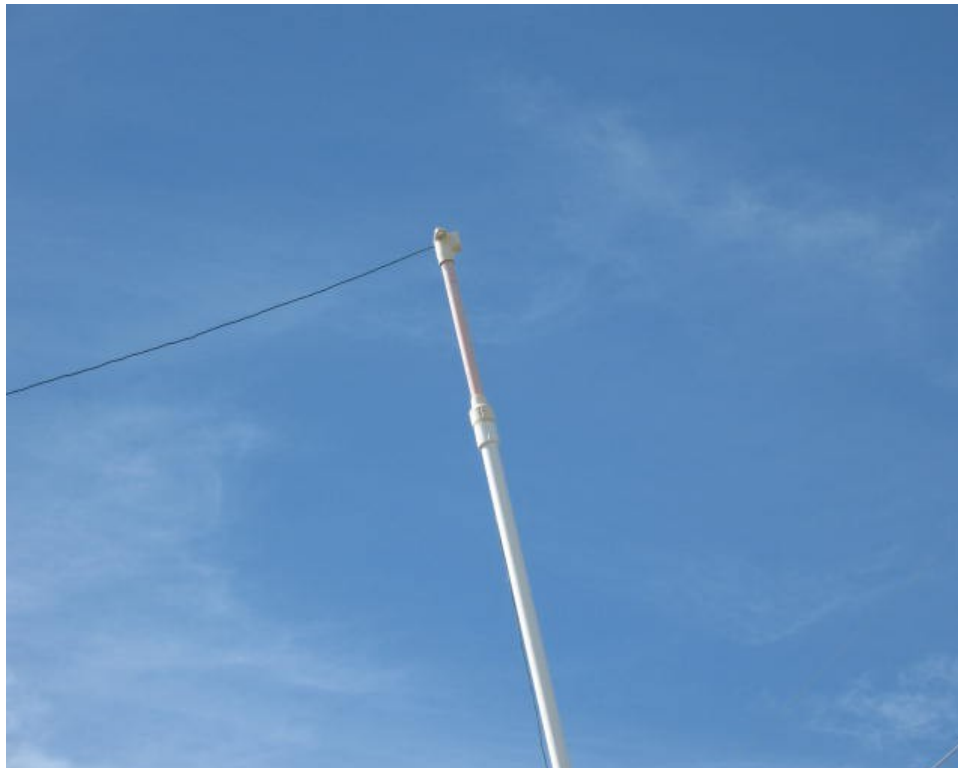
Note how a CPVC eared-elbow provides easy transition from vertical to flat-top on Q'nD inverted "L" antenna. (NZ1D photo)
