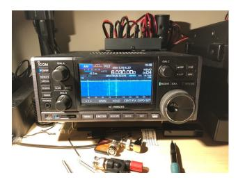
The IC-R8600 is a wide-band receiver, covering 10KHz to 3GHz, and can demodulate FM, AM and CW/SSB, as well as several digital modes, though I have not yet experimented with those. QST has a review in their November 2017 issue.
