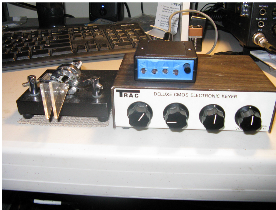
Illustration 2: Not your father's keyer: Ham Gadget's Ultra Picokeyer (on top of Charlie's vintage Trac keyer) provides a nice adjunct for the tiny Cricket QRP rig. (KT11 Photo)
