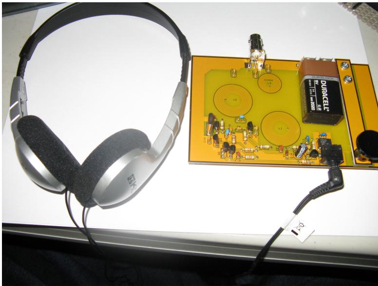
*Illustration 5: 500 mw on 80 meters; KT1I's Cricket QRP Transceiver*
