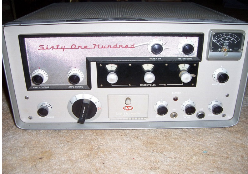
B&W 6100 Transmitter, one of the first ham radio transmitters employing frequency synthesizing
