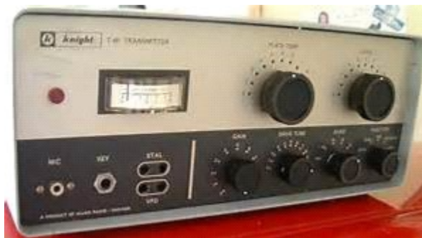
Knight-T60, a 4-tube, 80-10 meter, 60 watt AM/CW transmitter. (W1HFN photo)
