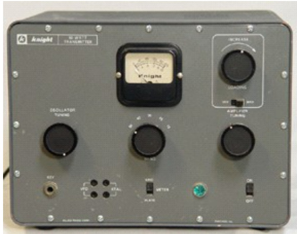
Knight Kit T-50, a 3-tube, 80-10 meter, xtal controlled 50 watt CW transmitter aimed at the Novice licensee. (W1HFN photo)
