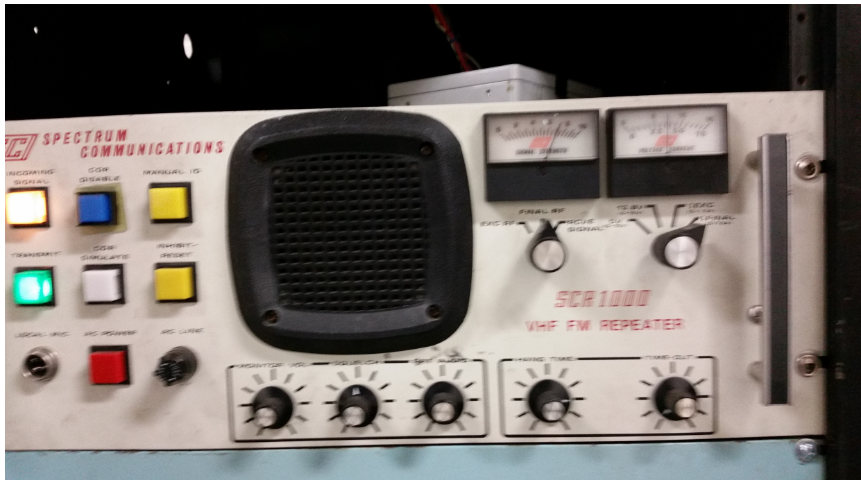
WIGZ repeater front panel showing relative power of final at 42 watts (left-hand meter) and final current at approximately 7.5A (right-hand meter)
