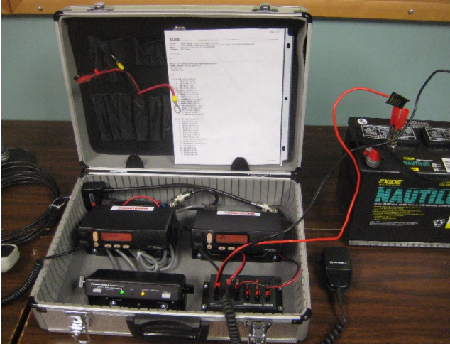
above: Bill N1UZ displayed a 40 watt portable 2m/70cm crossband repeater he built using Motorola radios. kd1sm photo
