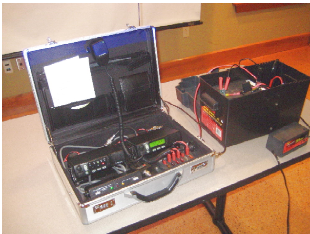
Above: At the February MARA meeting John N2YHK, ARRL Western Massachusetts Section Emergency Coordinator, displayed a portable 2m/70cm repeater constructed by the Worcester Emergency Communications Team. [kd1sm photo]
