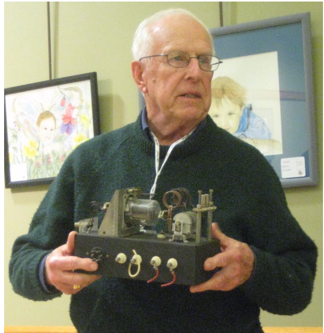
Above and below: Tom K1JHC shows a single-tube 829B receiver.
