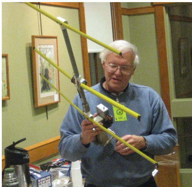
Above: Barry W1HFN shows his fox hunting gear, including the 'tape measure beam'.
